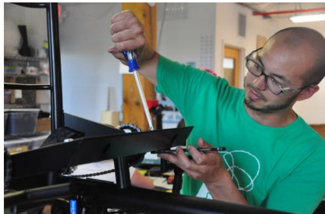
(b) Use a #3 (or any available) Philips screwdriver and a 13mm wrench or socket to loosen the bolts.
