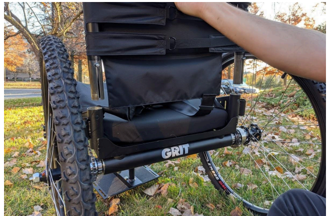
c) Continue pulling upward on both sides of the seatback until it is released.
