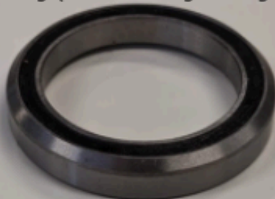
#7: Bearing (note the angled edge)
