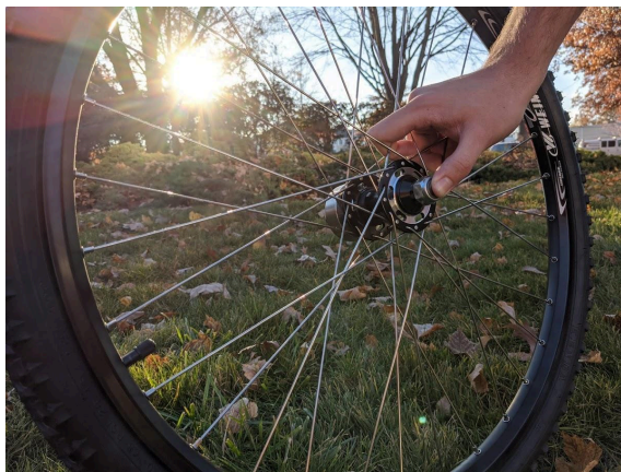
a) Press the quick-release button on the axle inward.
