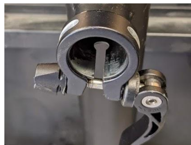
e) Slide the clamp back onto the frame.
