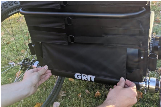
a) Slide the seatback into the receiving sockets on the back of the seat. Keep the seatback level while you slowly insert it into the sockets.
