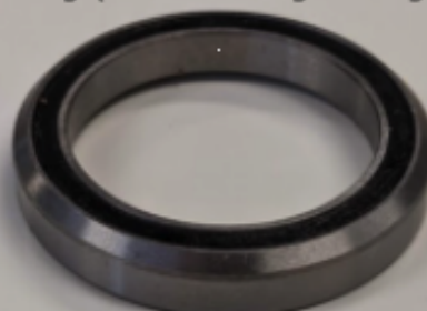
#8: Bearing (note the angled edge)
