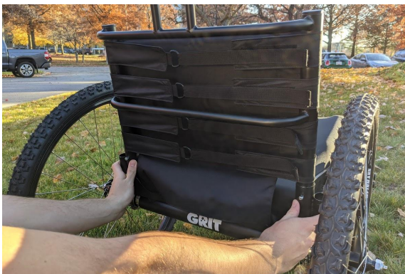
c) Slide the seatback down until the push buttons pop out on both sides.
