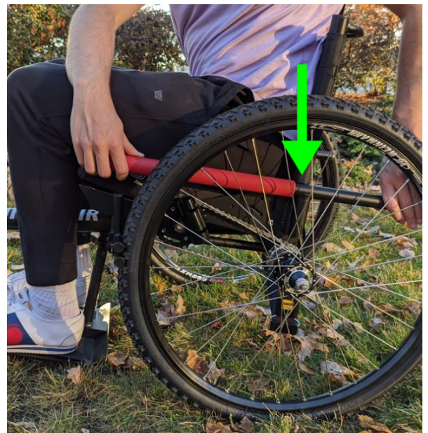
d) Insert the brake into the lever holder.
