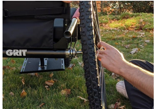
b) Align the axles with the axle receiver.
