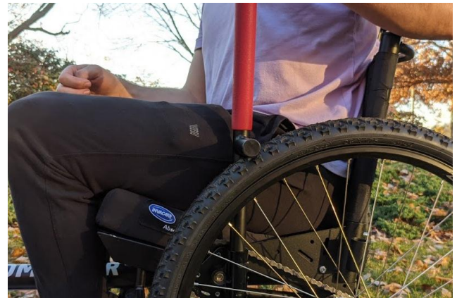
d) Make sure the brake is over the wheel and that it doesn't rotate when the lever is pulled back.
