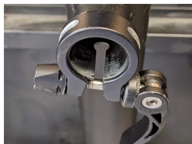
e) Slide the clamp onto the frame.
