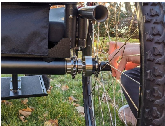
c) Align the grooves on the coupling and insert the axle.
