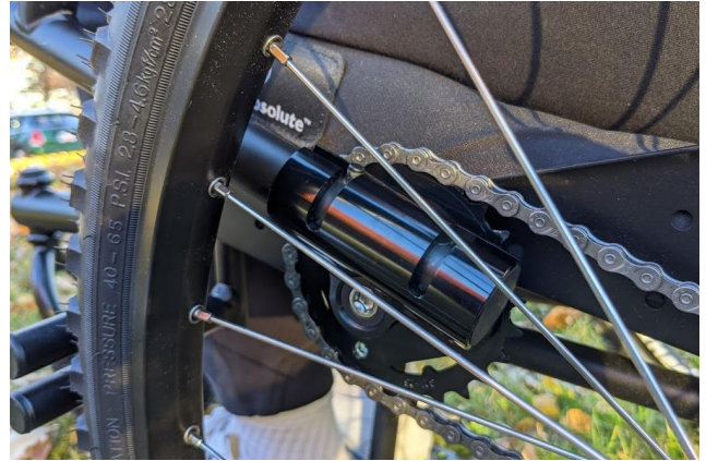
b) Insert the lever into the coupling hole until the pin reaches the bottom of the slot.
