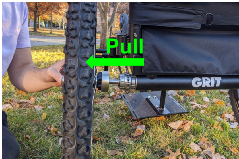
b) Pull the wheel straight away from the chair while keeping the button pressed.
