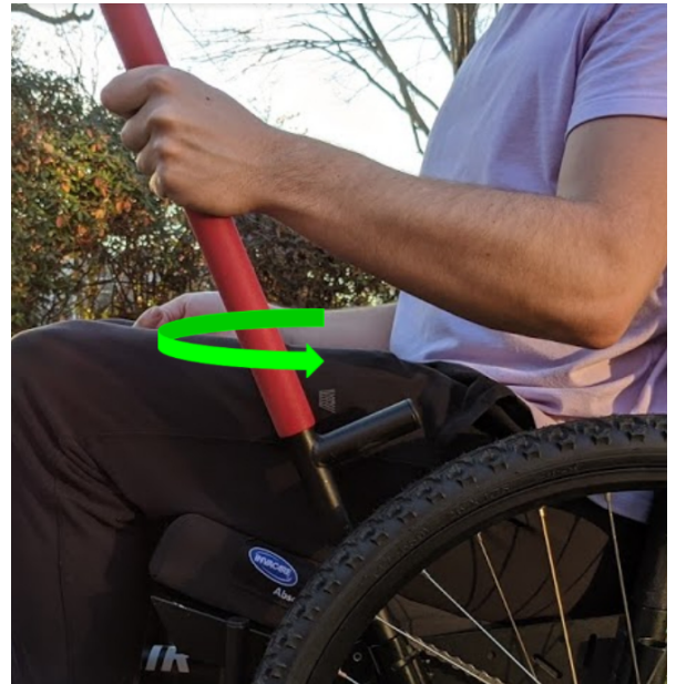
b) Rotate the brake bar toward yourself.
