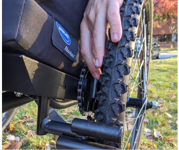
b) If the lever hole is inaccessible, rotate the coupling.
