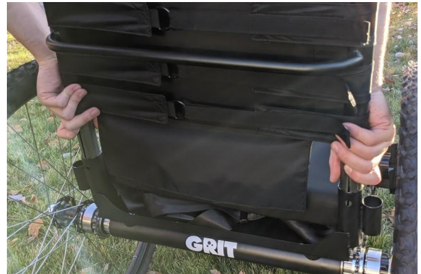
b) With your fingers, push the spring buttons inward on both sides of the seatback while lowering the seatback into the seat.
