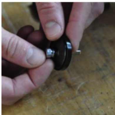
g) Insert the screw with the split washer through the hole in the top cap. Grab the top cap, spacer, and screw in your hand.
