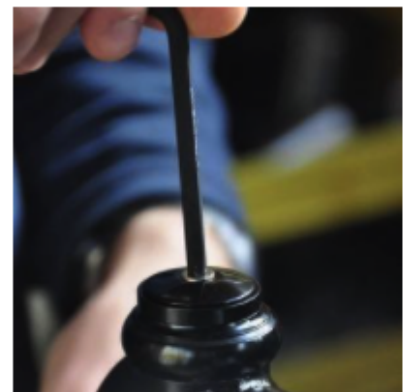
i) Tighten the screw with the provided Allen key until you start to feel resistance when rotating the fork left to right.
