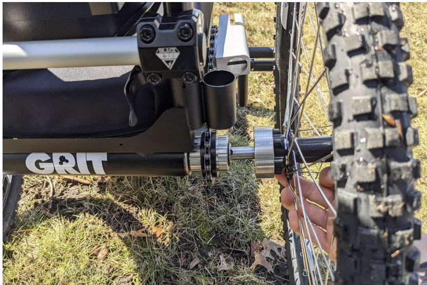
b) Pull the wheel straight away from the chair while keeping the axle button pressed.
