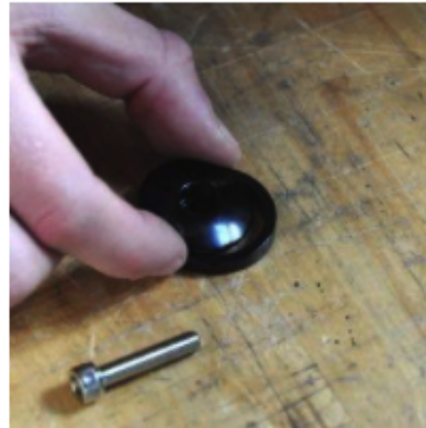
e) Put the top cap, cone side down, over the spacer.
