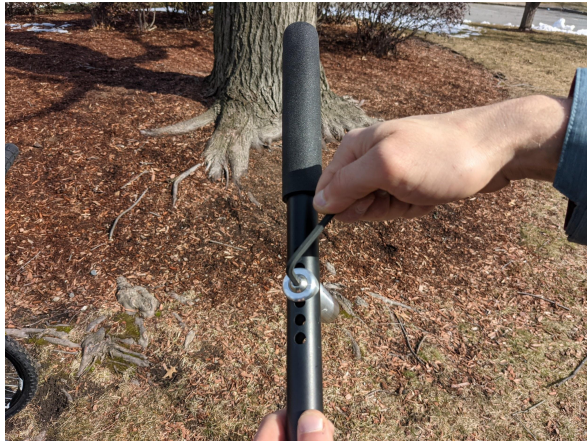
a) Use a 5mm Allen key to begin loosening the brake bar bolt.
