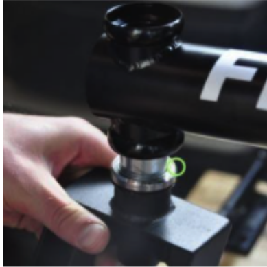
a) Slide the bearing onto the fork, curved (chamfer) side up. Push the fork tube into the Freedom Chair.
