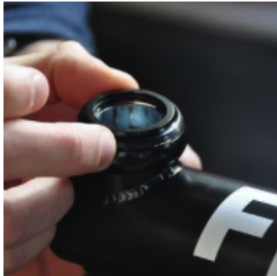
d) Slide on the bearing cover, flat side down.
