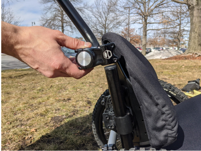
c) Slide the Trail Handle clamp over the seatback cane. NOTE: For the lowest-profile setup, the grips of the Trail Handles should face outward (away from each other).
