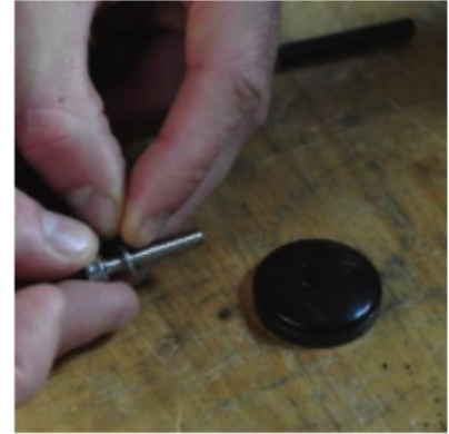
f) Slide the split washer onto the screw.
