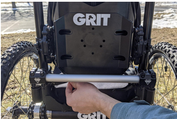
c) Fasten the clamps on both sides to secure the seatback in position.
