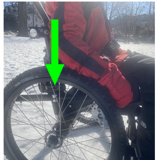
d) If desired, store lever in the holding sleeve.
