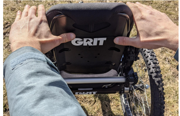
b) Push the seatback down on both sides to lower it farther into the sockets.
