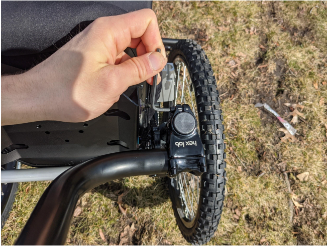
e) Tighten the inward-facing bolt on the Trail Handle clamp.
