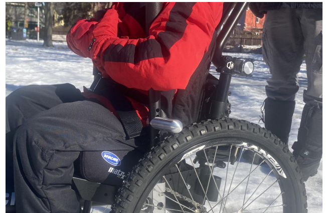
d) Make sure the brake is over the wheel and that it doesn't rotate when the lever is pulled back.
