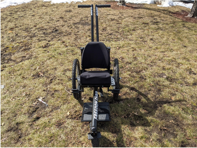
f) Repeat steps b-e for the other handle. Above is the final product, with both Trail Handles installed.
