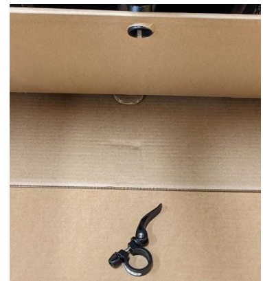
c) Slide off the clamp to free the frame.
