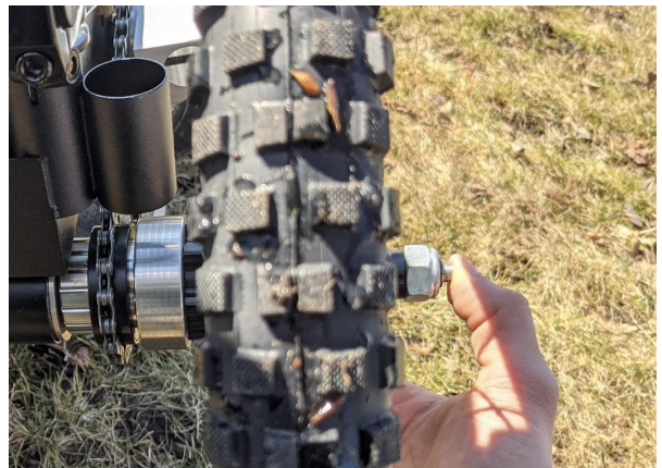
d) Ensure the push-button on the axle is out and the coupling is fully attached.
