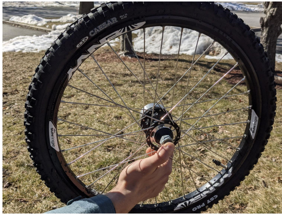
a) Press the quick-release button on the axle inward.
