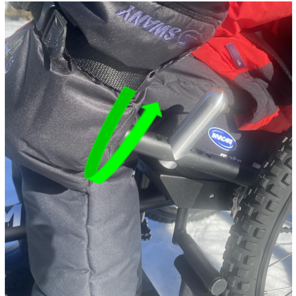
b) Rotate the brake bar toward the rider.
