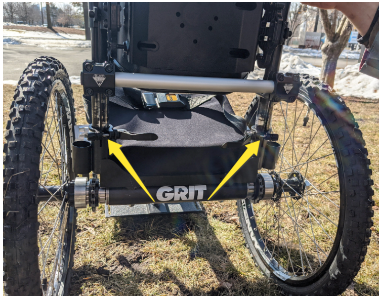
a) Loosen the bike clamps on both sides of the seatback
