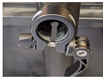
e) Slide the clamp onto the frame.
