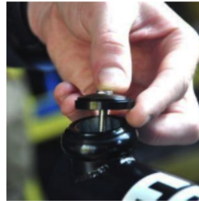
h) Put the top cap, spacer, and screw on top of the headset and thread the screw into the nut within the front wheel fork.
