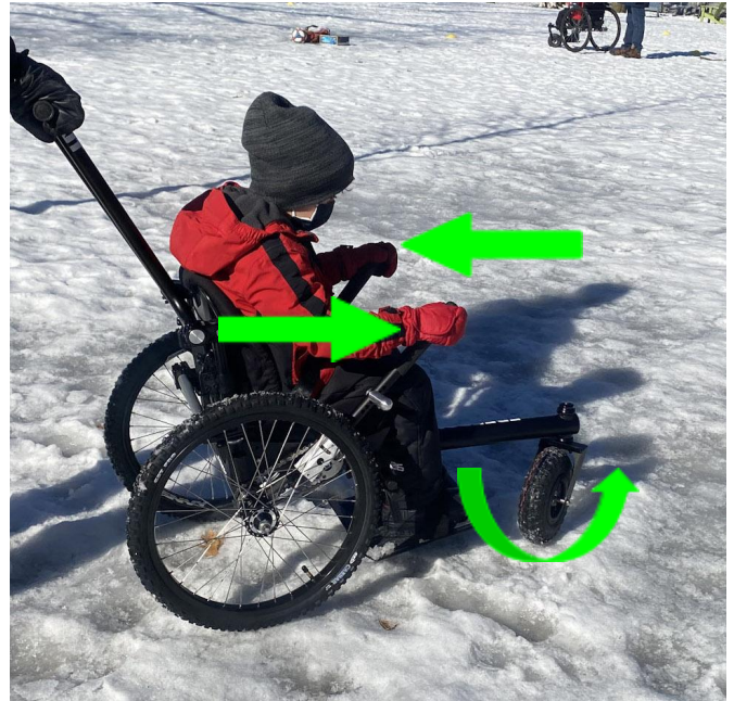
b) To turn left, apply the brake with the left lever and push the right lever forward.
