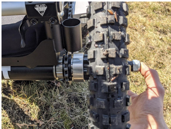
c) Align the grooves on the coupling and insert the axle.
