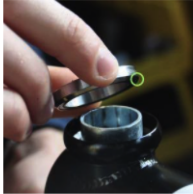
b) Slide on the top bearing, making sure the curved (chamfer) side of this bearing is facing down toward the ground.
