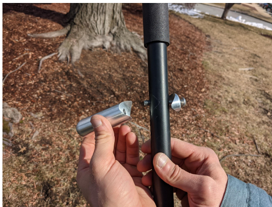
c) Fully remove the brake bar.
