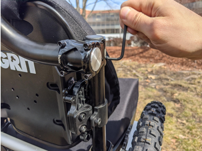
d) Tighten the outward-facing bolt on the Trail Handle clamp.
