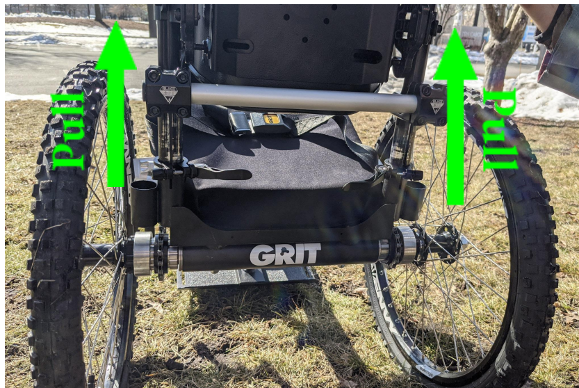
b) Pull upward on both sides of the seatback until it is released.
