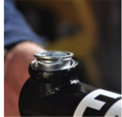
c) Slide on the compression ring, cone side down, as far down as you can. It doesn't matter which direction the split is pointing.
