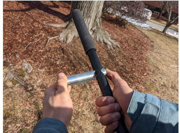
b) Once the brake bar is loose, finish removing it by hand-loosening the brake bar.
