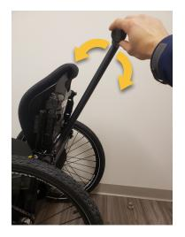
Retighten the four bolts on the Trail Handle receiving clamp.
