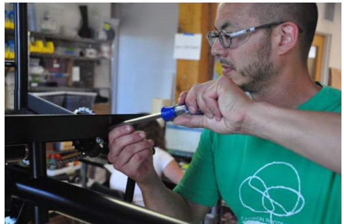
(d) Use a #3 (or any available) Philips screwdriver to tighten the setscrews until the desired chain tension is reached.
