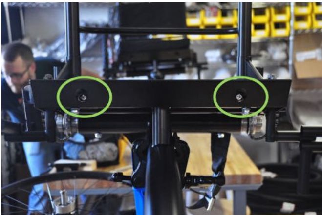
(c) The chain tightness is controlled by two setscrews, one on each side of the seat. Both must be rotated the same amount.
