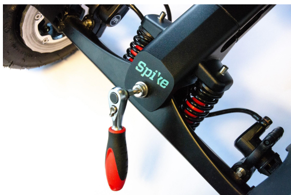
Figure 4.1.2 - Tightening steering system
