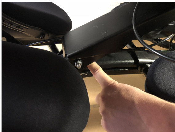
Figure 6.4.1 - Danger of trapping fingers during folding.
