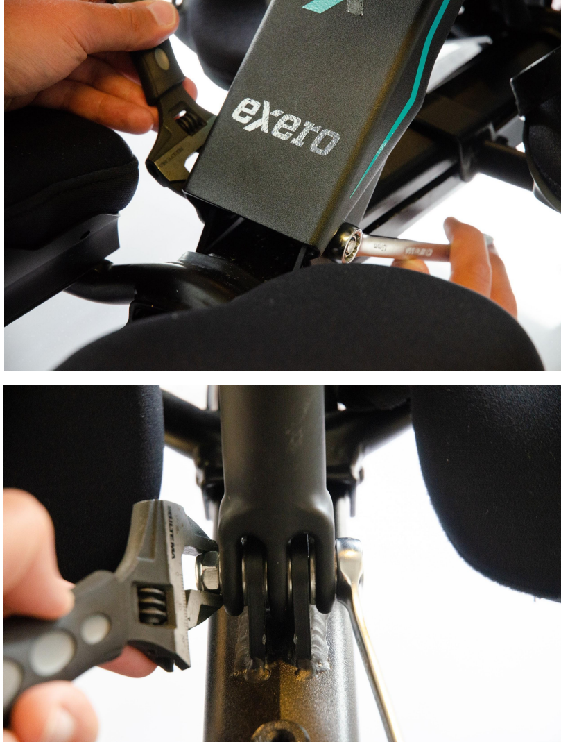
Figure 4.1.3 - Tightening seat arm (right) and seat post (left)
