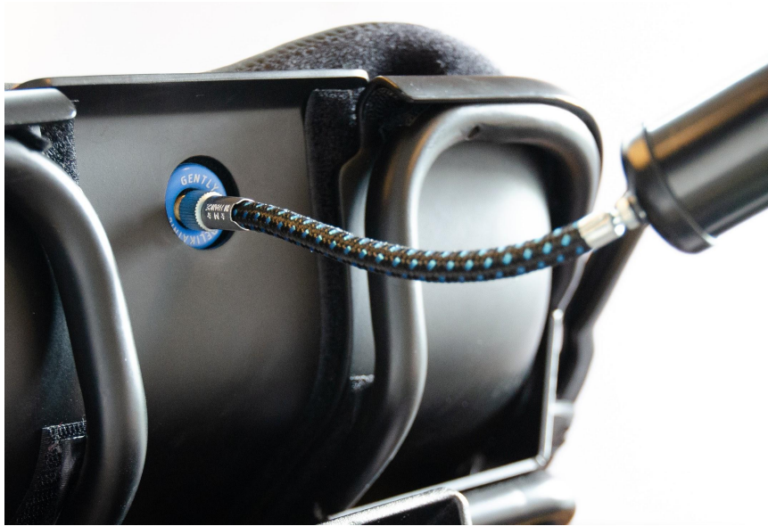
Figure 3.4.12 - Pump and adapter mounted for draining air.
