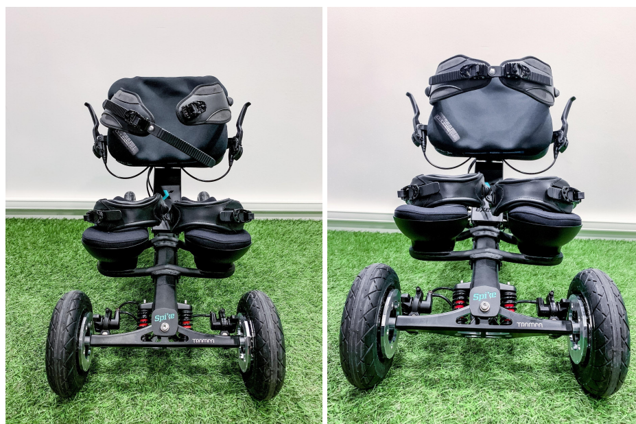
Figure 3.4.12 - Hip strap in open and closed position
