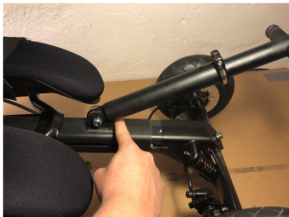
Figure 6.4.1 - Danger of trapping fingers during folding.
