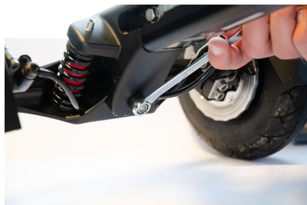
Figure 4.1.2 - Tightening steering system
