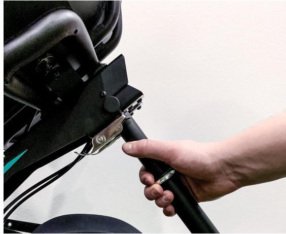
Figure 3.4.5 - Risk of trapping fingers
